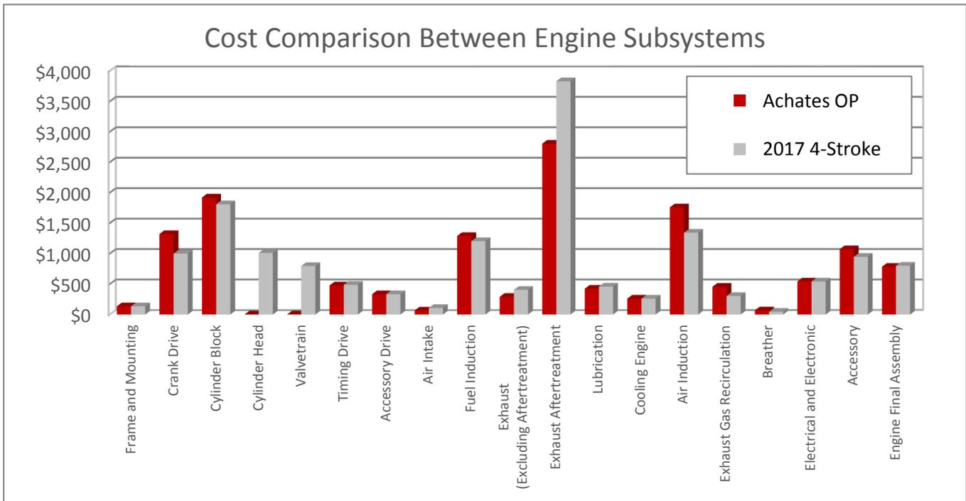
Figure 2: Engine Subsystem Cost Comparison
