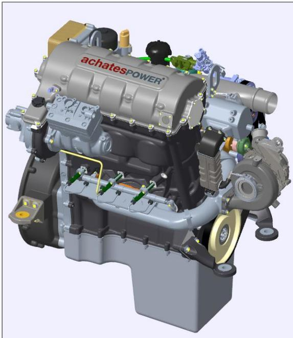
Figure 1: CAD rendering of 7.9L Opposed-Piston Engine
