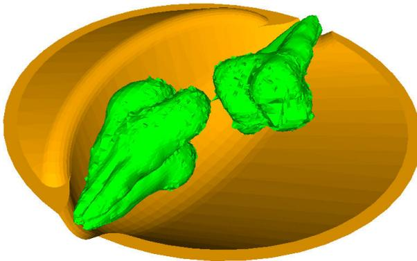
Figure 4: Schematic of the combustion system with plumes coming out of two side-mounted injectors.
