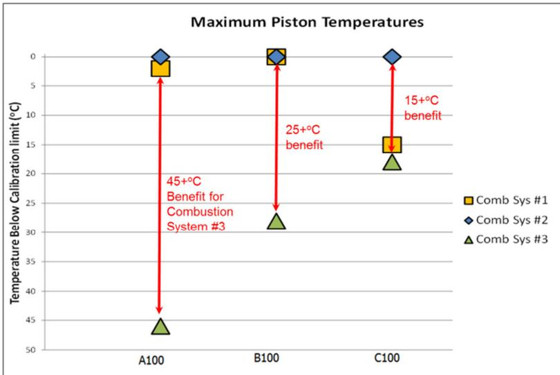
Figure 8: Maximum measured piston crown temperature for different combustion systems.
