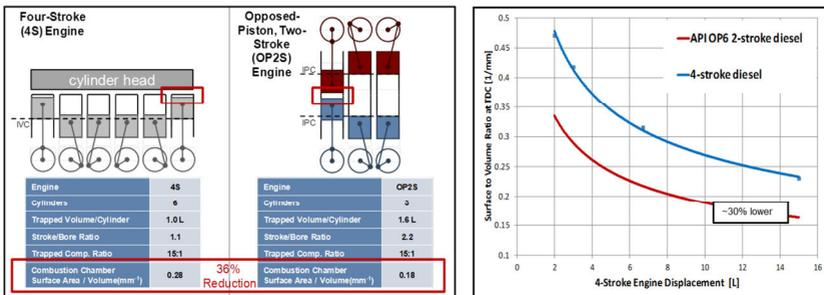
Figure 1: Combustion chamber surface area versus volume comparison between OP2S and conventional four-stroke engines.
