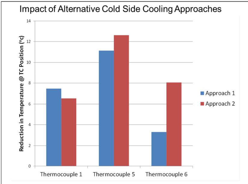
Figure 9: Impact of alternatives on piston under-crown cooling.
