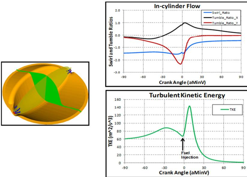
Figure 5: In-cylinder charge motion in an OP2S engine.
