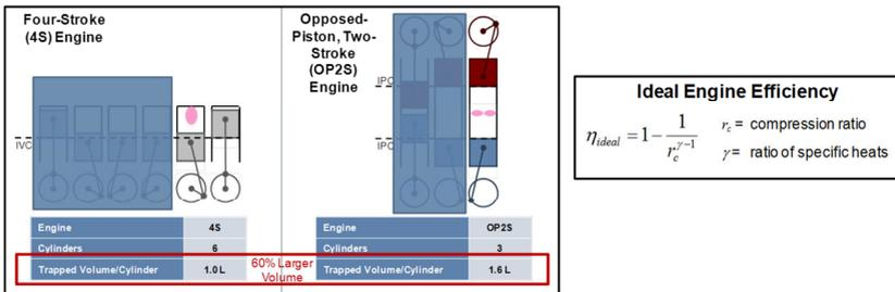
Figure 2: Illustration of leaner combustion in an OP2S.
