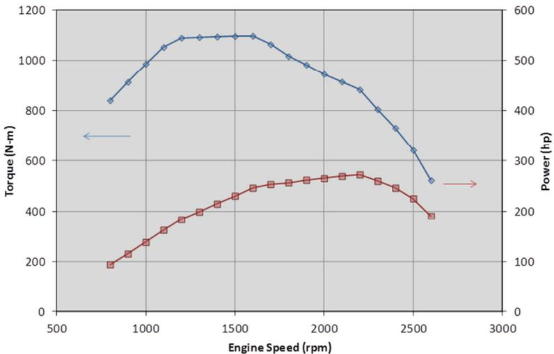
Figure 15: Torque and power curve for the 4.9 L three-cylinder engine.
