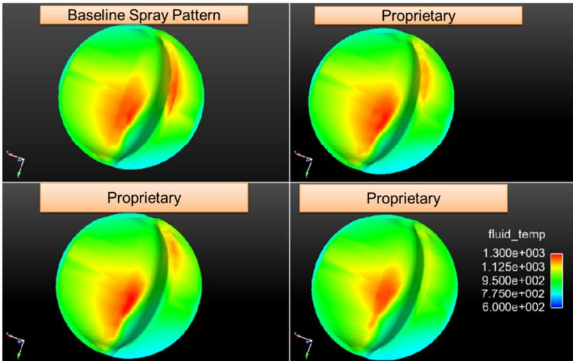
Figure 7: Effect of spray patterns on near-wall fluid temperatures.
