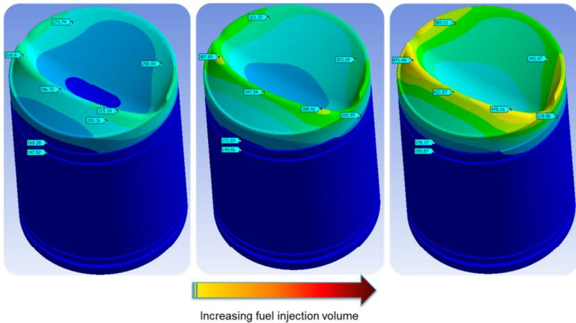
Figure 6: Effect of engine load on piston crown temperatures.
