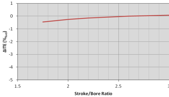
Figure 3: Effect of Stroke/Bore Ratio on Indicated Thermal Efficiency
