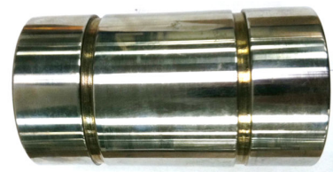
Figure 13: EMD710 Bi-axial Wrist Pin with 18,000 Hours in Service
