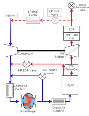
Figure 1: Air Path Schematic
