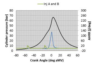
Table 6 Mode 8 cylinder pressure, AHRR and injector current traces
