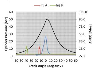
Table 5 Mode 1 cylinder pressure, AHRR and injector current traces
