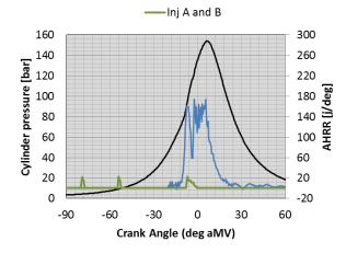
Table 7 A75 cylinder pressure, AHRR and injector current traces
