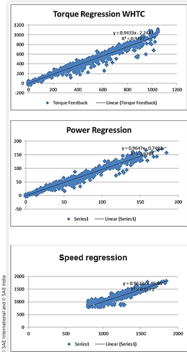
**FIGURE 6** Conformance of multi-cylinder OP Engine to WHTC regulatory cycle
