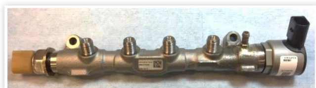
FIGURE 22 Fuel rail with rail pressure sensor (RPS) and high-pressure valve (HPV).
