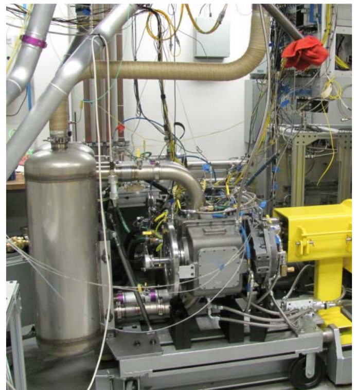
Figure 8 . Single-cylinder research engine installed in test cell.
