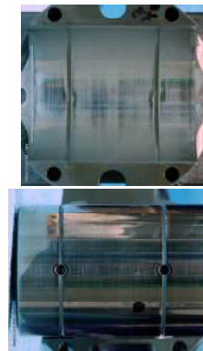
Figure 14: A48 1.6L SCE: Wrist Pins after 50 Hours Full Load Durability
