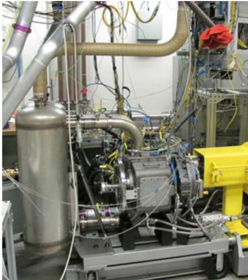
**Figure 2. Test cell setup of the single-cylinder research engine.**
