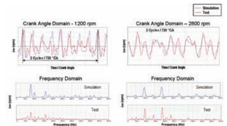
Figure 6: Correlation of Crank Nose Speed Fluctuation
