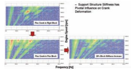
Figure 2: Support Structure Sensitivity, Influence on Crank Bending
