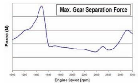
Figure 3: Maximum Gear Separation Force Over Engine Speed
