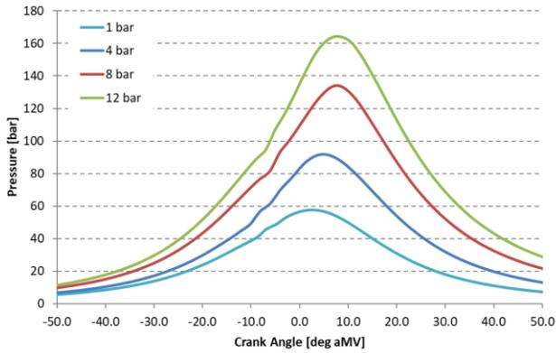
Figure 4 Diesel cylinder pressure traces
