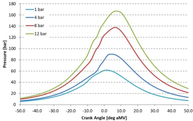
**Figure 2 GCI cylinder pressure traces**
