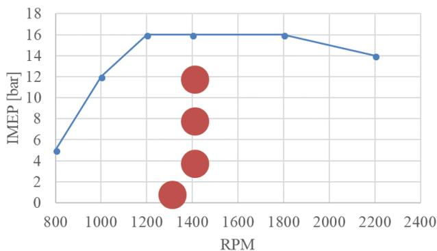
**Figure 1 GCI and diesel SCE test points**
