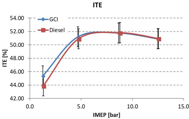
Figure 10 Indicated thermal efficiency
