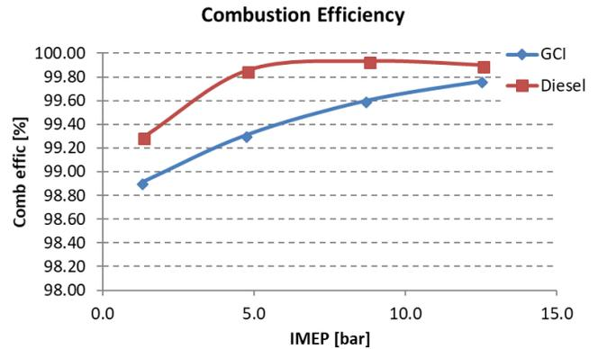
**Figure 15 Combustion efficiency**
