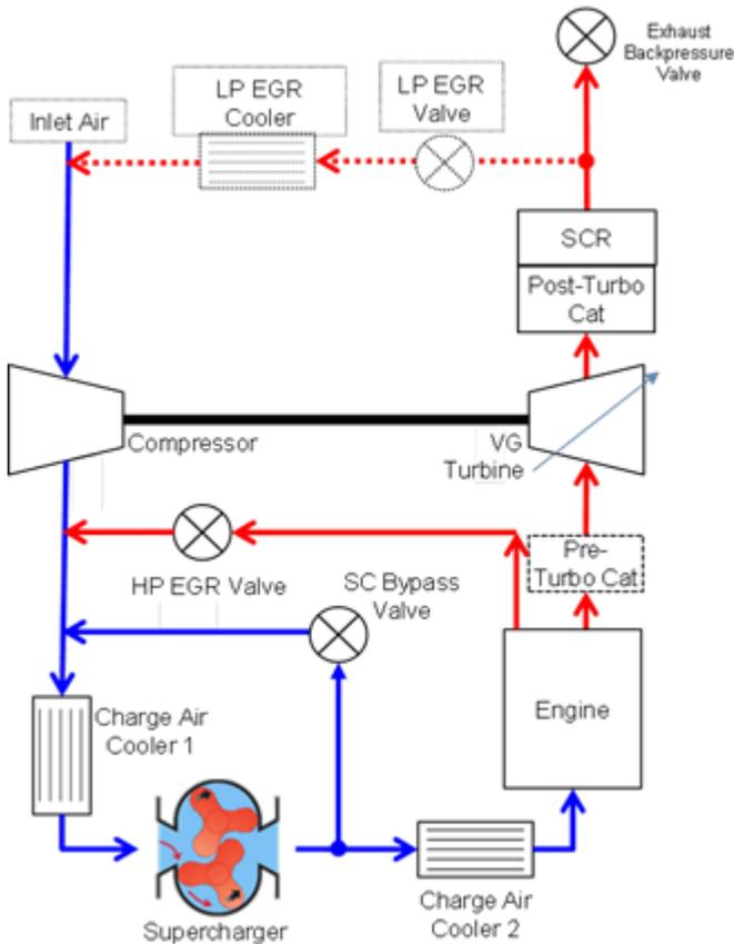
Figure 1: Air Path Schematic
