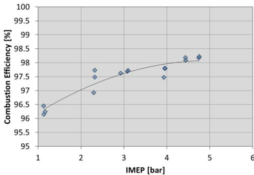
high-efficiency, low-load GCI operation possible with a greater than 96% combustion efficiency. This is achieved because of the high exhaust residual and enabled with practical hardware and fuels. (Tables 2, 3)
