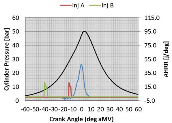
Table 5 Mode 1 cylinder pressure, AHRR and injector current traces
