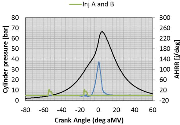
Table 6 Mode 8 cylinder pressure, AHRR and injector current traces
