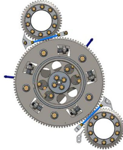
**Figure 3 OPGCI engine gear train**
