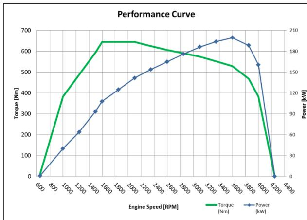
**Figure 2 OPGCI engine torque and power curves**
