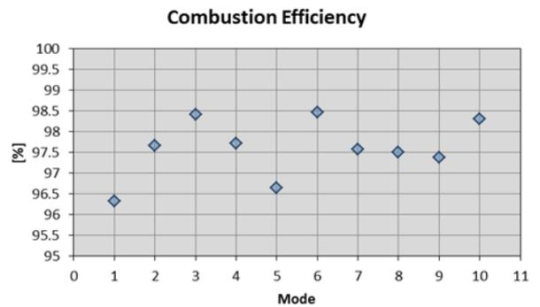
**Figure 8 Combustion efficiency of LD operating points on the 10 mode cycle approximation**
