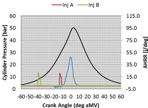
**Figure 10 Mode 1 cylinder pressure, AHRR and injector current traces**
