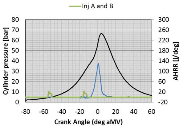
**Figure 11 Mode 8 cylinder pressure, AHRR and injector current traces**
