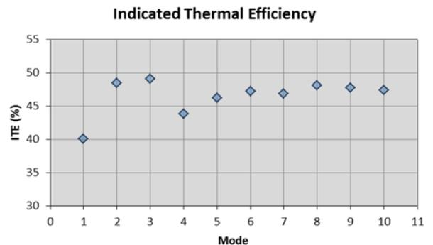
**Figure 9 Indicated thermal efficiency of LD operating points on the 10-mode cycle approximation**
