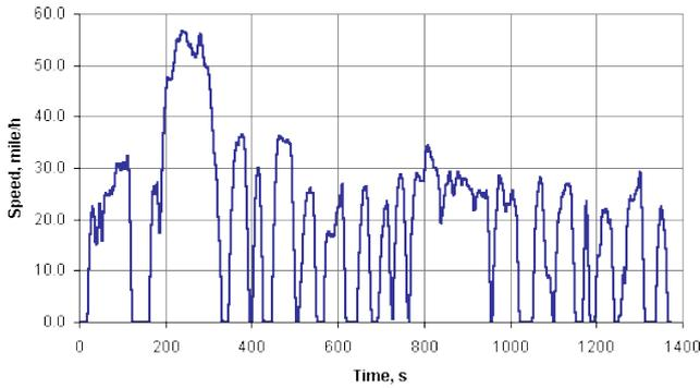
**Figure 4 US FTP75 Test cycle speed vs time [16]**
