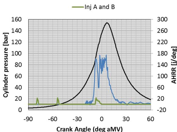
**Figure 12 High-load cylinder pressure, AHRR and injector current traces**
