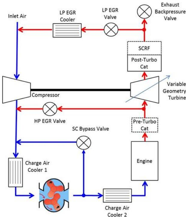
**Figure 5 OPGCI complete airsystem diagram**
